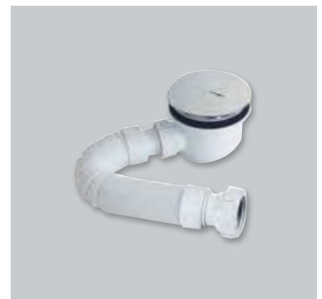
90mm Fast flow shower waste and flexi pipe 265-900mm (will fit tray up to 15mm thick)
